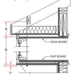
C. When the bay/bow unit is being installed, thread the threaded end of the cable through the "T" nut, down the length of the bay/bow unit, and through the drilled hole in the seat board. Place a washer and two hex nuts on each cable end.
